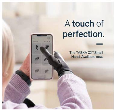
The new TASKA CX is the small hand destined to play a big role in your daily life. All fingers and thumb are capacitive touch capable, meaning they can be used on any common touch screen.
